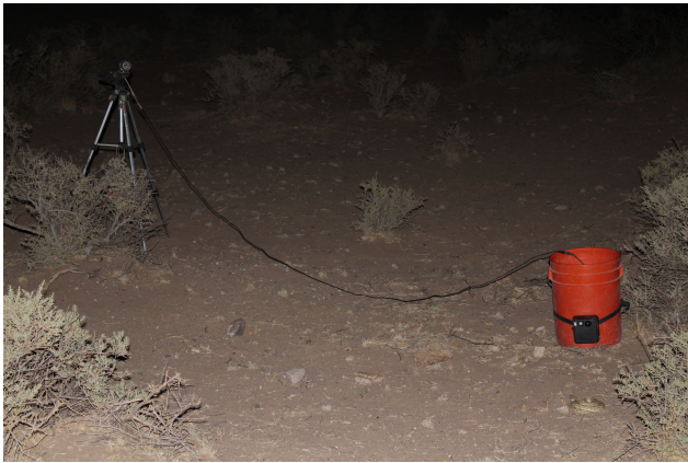
FIGURE A1 A typical example of the fixed-field videography unit used to study foraging ecology. The set-up consists of a near-infrared (IR)-sensitive surveillance camera mounted 1 m from a coiled snake, approximately 45° to the left or right side in front of the snake's head, followed by a separate IR light positioned around 3 m away from the front of the snake to illuminate a 1 m 2 area around the snake. This unit is recording a prairie rattlesnake ( Crotalus viridis ) with the snake in the lower right corner of the photograph.
